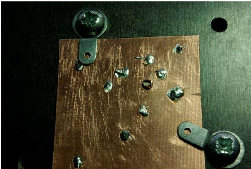
underside, smoothed off all edges, pretinned all copper surfaces top and bottom, applied plenty of flux and initially soldered the 24 pads - they looked good and I felt very satisfied at having done so.
