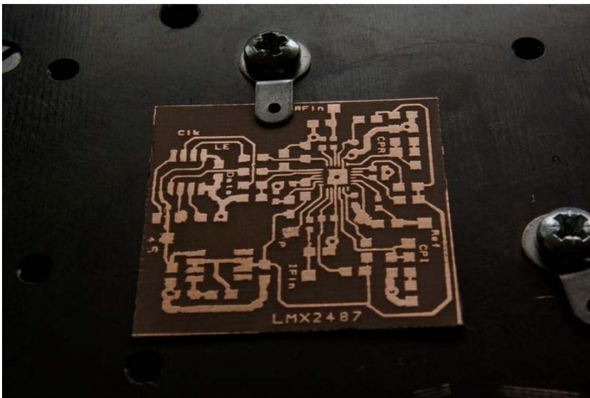
On the tiny 4mm square leadless packages many of the half-decent microwave synthesizers come in, the pad on the underside is only 2.5mm square. For the first one of these for which I tried to make a homebrew PCB, I drilled a 2.3mm hole (which was a bit too large, see photo) on the
