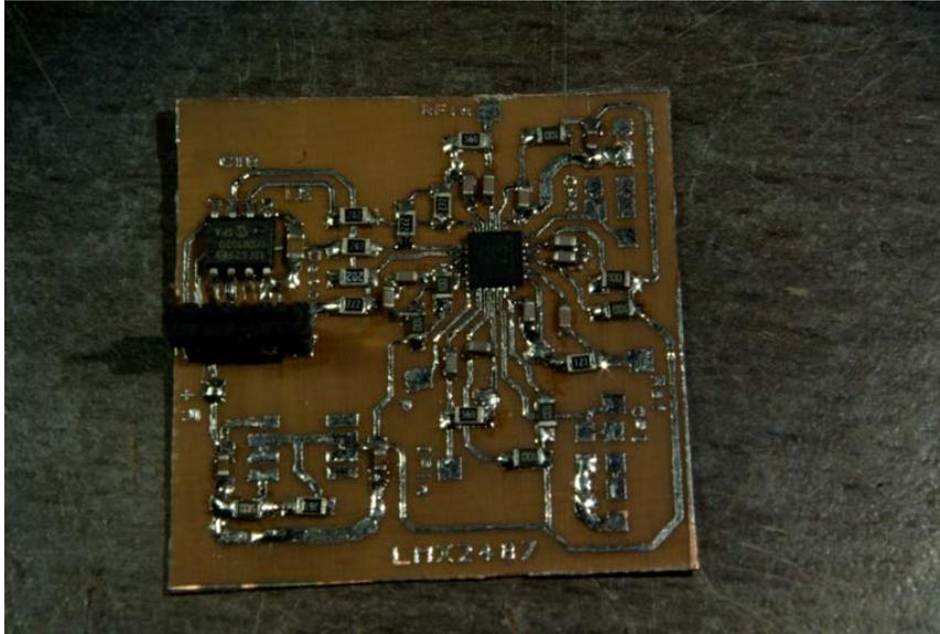
awful lot of heat. Realisation struck. The top of the IC pressing onto the metal surface was conducting heat away too rapidly. For the next time I placed three thicknesses of paper between the top of the IC package and the metal to act as a heat insulator. Soldering the pad was now much easier.
