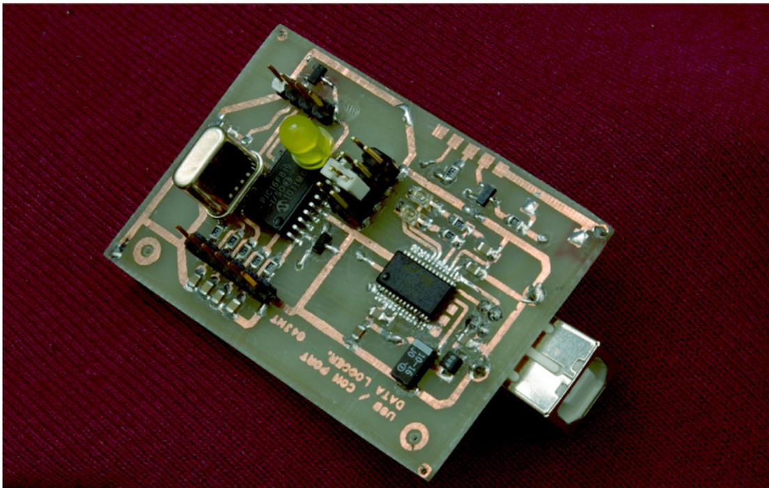
Prototype homebrew version of the 60 x 40mm PCB, showing the full USB enabled HF 10 data Logger. Analogue connections are made to the header on the bottom left of the photo. Measurement interval and output format by selecting the links on the dual header in the middle of the board. Top left is the in-circuit programming interface. For the COM-port only version, a 9 pin D socket can be mounted on the edge of the board, using the pads on both sides of the PCB, shown top centre.
