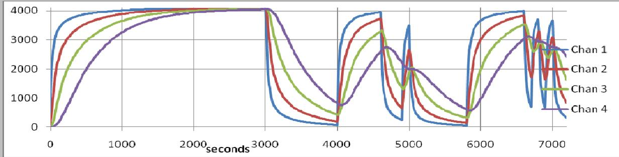
An example of the sort of plot that can be generated by the HF-10 Data Logger. All four input channels read the voltages on each capacitor of the circuit below as the switch was repeatedly changed over. The output data was saved to a file using *Hyperterm* on a host PC; the file then read directly into an Excel spreadsheet to generate the plot.
