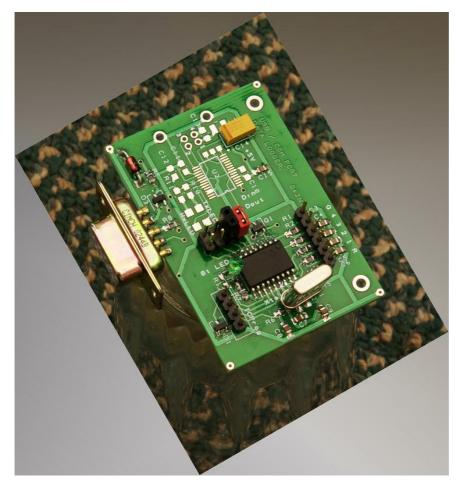
The Pads on the side of the board are designed to connect directly to a 9 Way D-Type female socket. It may be a bit tight, especially if a second-hand connector has been used with solder on the tags.
