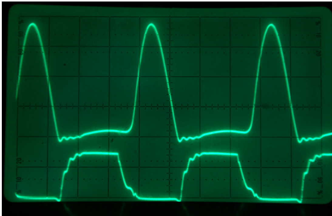
Photo 2 - Switching Waveforms. Top - Vdrain 50V/div. Bottom - FET Drive 10V/div
