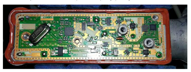
The PLL/Mixer chip is RDA3560m; a short data sheet can be obtained from <a href="http://www.uhf-satcom.com/misc/datasheet/RDA3560m.pdf">http://www.uhf-satcom.com/misc/datasheet/RDA3560m.pdf</a>
