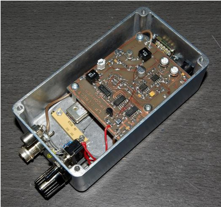
LF Upconverter PCB mounted above the RF source (based around an AD9850 DDS chip).
