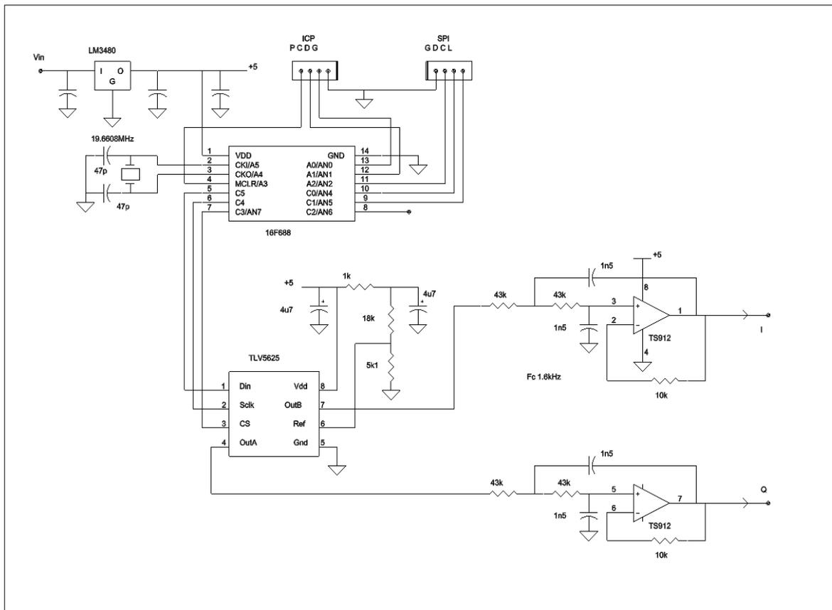
Figure 2 Baseband DDS generating I/Q frequencies in the range -1000 to + 1000Hz
