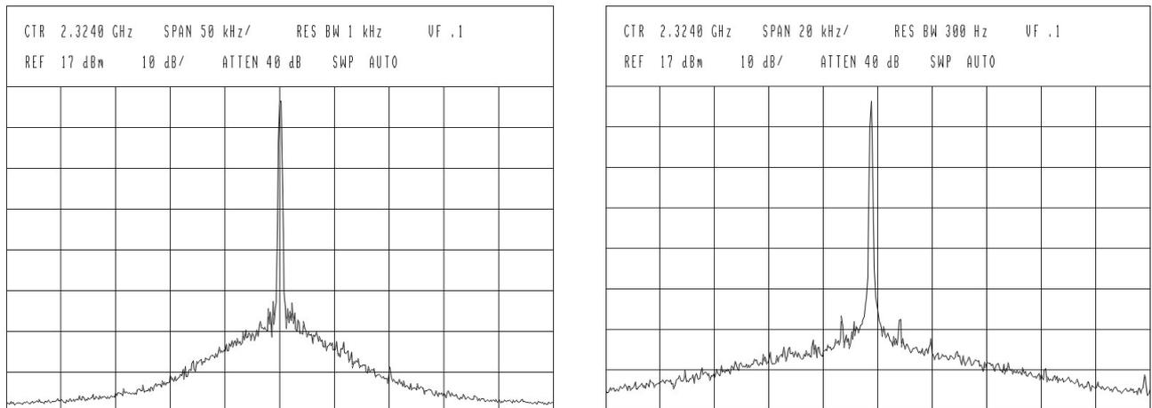
Figure 3 Phase noise of ADF4351 Source at 2.3GHz using a Leo-Bodnar GPSDO as a 10MHz reference input.
