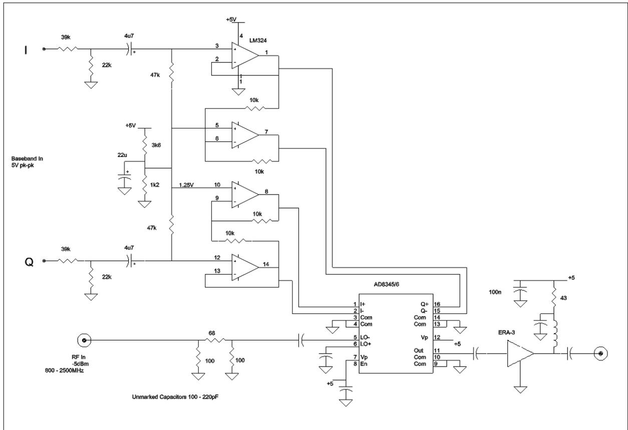
Figure 1 ADF8446 Quadrature upconverter with single ended to differential drive circuitry
