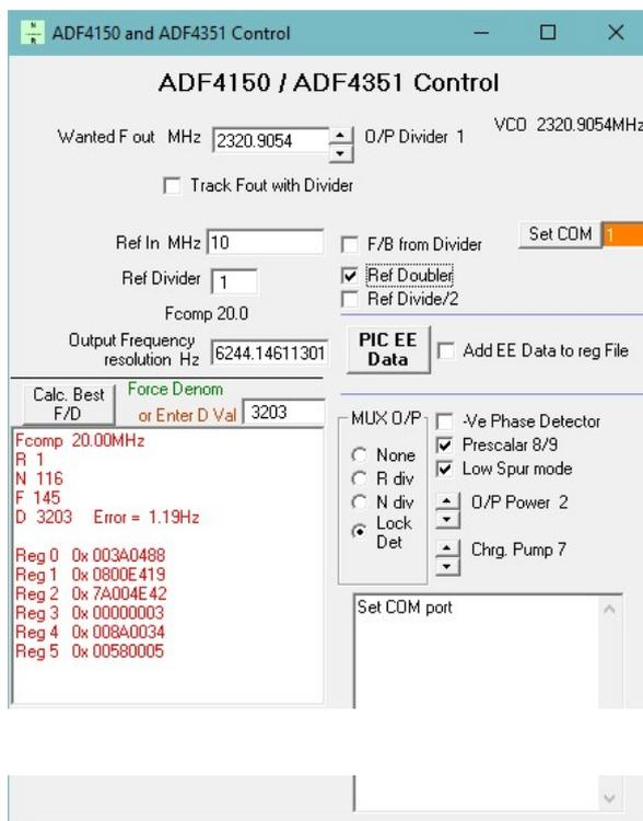
Figure 5 ADF4351 Register set finally adopted for best overall phase noise at 2.3GHz
