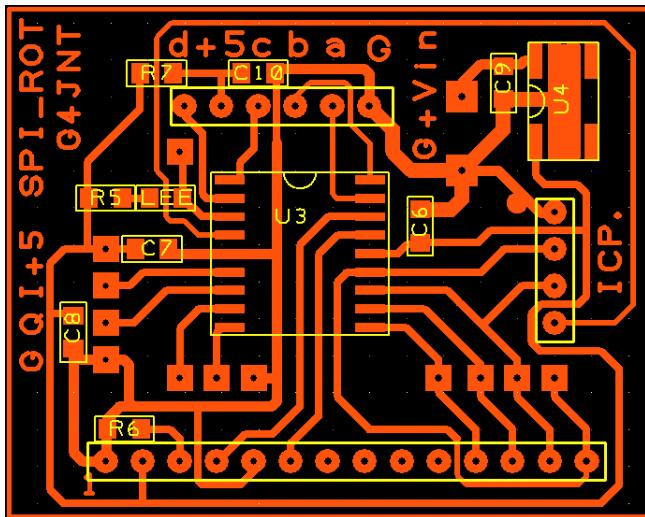
A PCB layout for SOIC packaged 16F628A PIC devices is shown below. The 14 pin header plugs directly onto the LCD modules available from [1], with all other connections made via pads or headers. Construction should be self explanatory. The LED serves no useful purpose in this design and can be left out. It is a hangover from an earlier project that used this PCB. (The odd pin connections for the serial interface to the DDS module are also a legacy of backwards compatibility)
