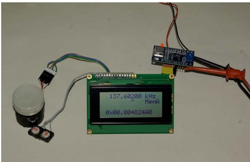
The tuning step, corresponding to each pulse from the rotary encoder, can be cycled through each decimal digit from 100kHz steps down to 0.01Hz by pressing the S pushbutton repeatedly. The digit being changed is shown by the caret on the second line of the display. Holding the S button down for 2 seconds stores the displayed frequency in the current
