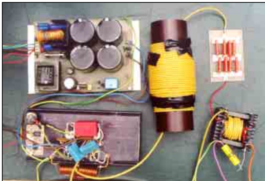
Fig 5—Transmitter components used for breadboarding: top-left, dc power supply; right-hand side, tank components and output matching / isolation transformer; bottom-left, driver and switching components.
