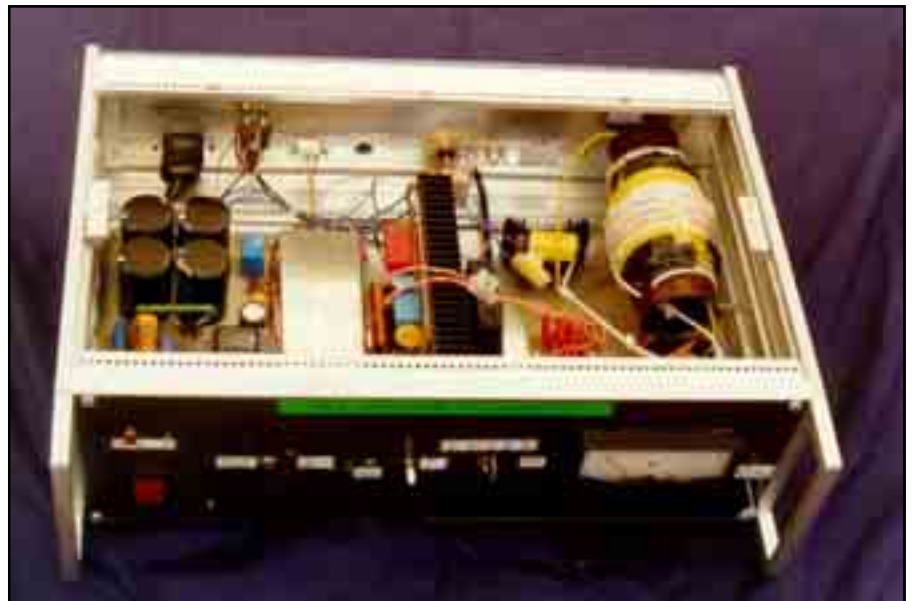
Fig 7—A close-up view of the active switching components.
